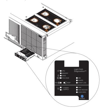
The system-error LED on the operator information panel is lit when certain system errors occur. If the system-error LED on the server is lit, one or more LEDs inside the server might be lit. Use the Light Path Diagnostics panel to identify the type of
